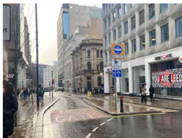
Camera controlled modal filter allowing access for buses and taxis
