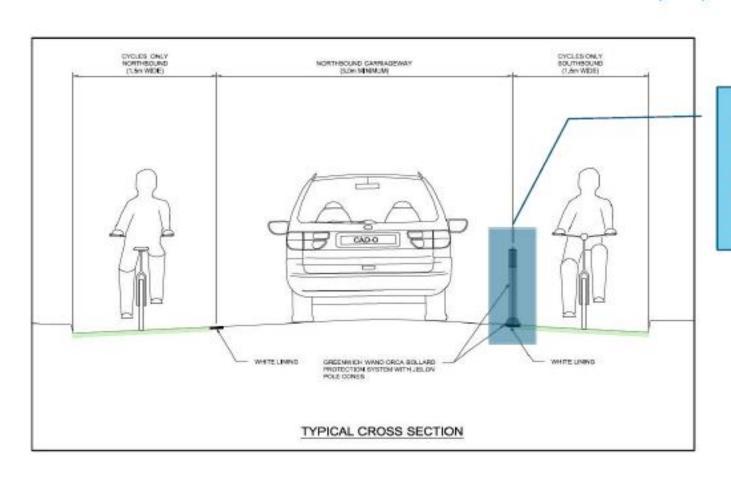
Location for installing removable separation. (currently showing Greenwich Wand Orca system as proposed by the scheme)
